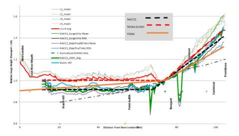
Figure 5Peak surge water level vs distance from New London , CT along the southern<br/>RI coast line, and up the central axis of Narragansett Bay relative to<br/>Newport, RI for NOAA SLOSH and ACOE NACCS simulations. Results are
